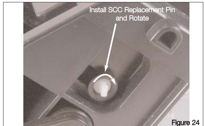
Install SCC replacement pins.
