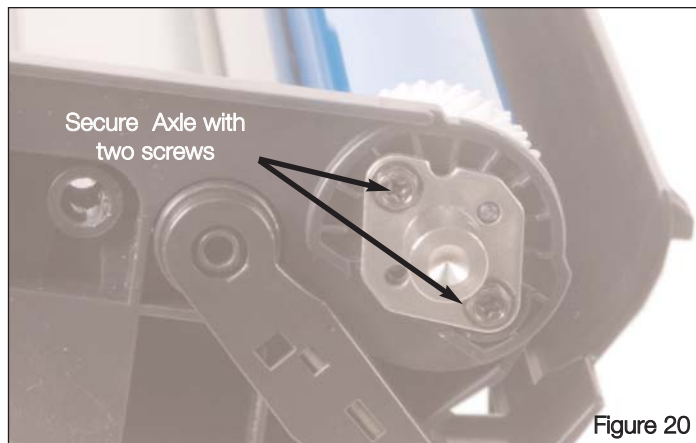
Secure the metal Drum Axle to the Drum.
