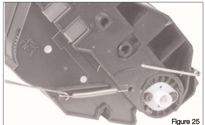
Attach the tension spring to the Contact side of the cartridge.
